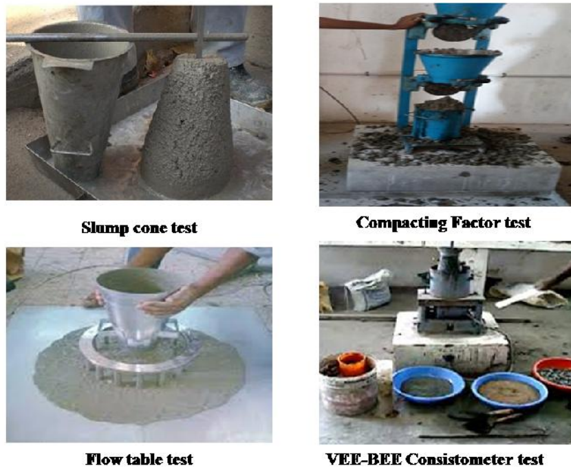
Figure 4.1 Slump Cone Test, Compacting Factor test, Flow Table Test and Vee-Bee Consistometer Test
