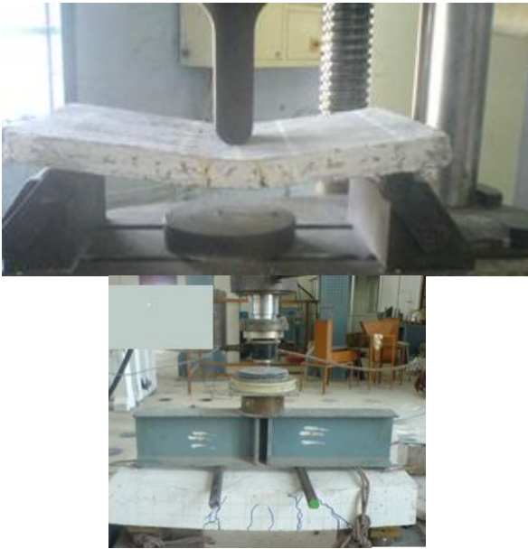
Fig No. 8 Test setup of ferrocement panel and RCC Slab
